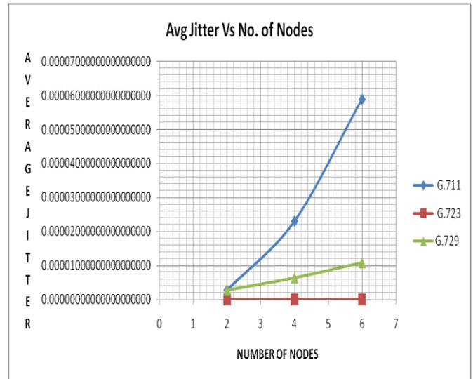
Fig. 3 Average jitter for various VoIP codecs
