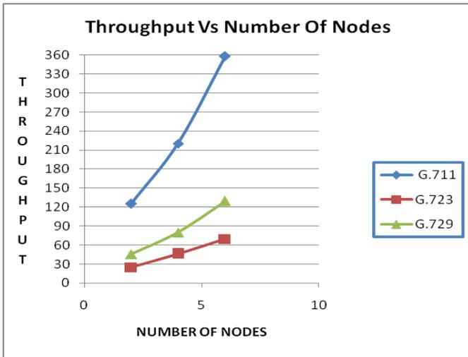
Fig.2 Throughput for various VoIP codecs
