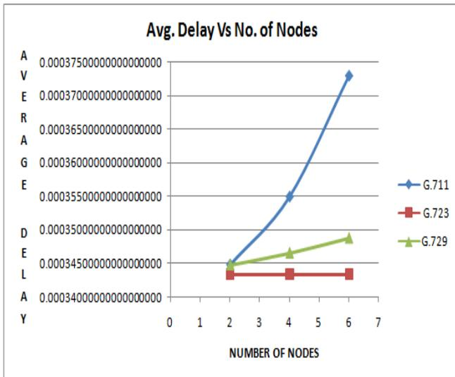
Fig. 4 Average Delay for various VoIP codecs
