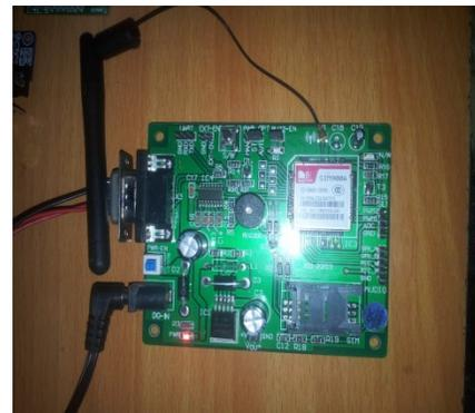
Fig. 6- GSM Modem
