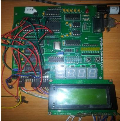
Fig. 3- NXP89V51 microcontroller board.
