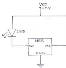
Fig. 4- Hall Effect sensor with LED
