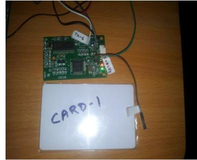
Fig. 5- RFID reader/writer module
